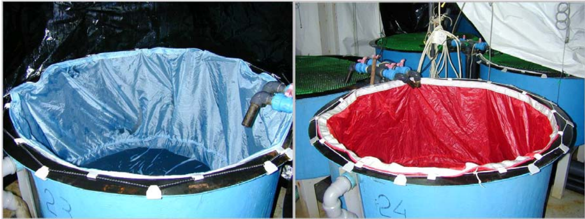
Figure 6. Tank system and textile bags manufactured for the needs of the project and used as background colour in Experiment 3.
